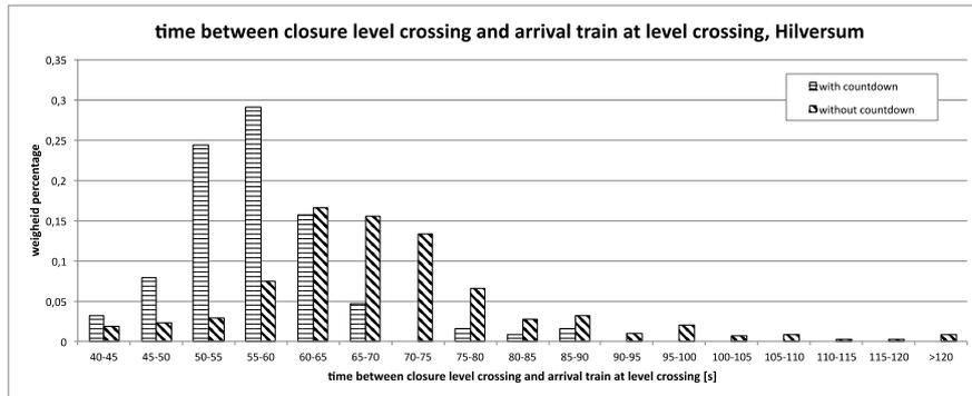
**Figure 2: Time between closure of level crossing and arrival of the train at the level crossing, with and without countdown**
