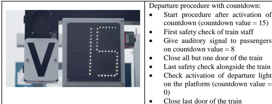
**Figure 1: Final countdown device with deactivated departure light and procedure of departure of the train**
