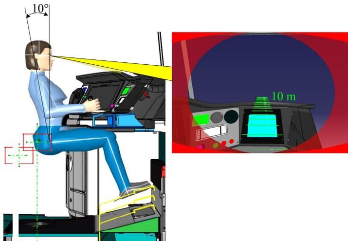
**Figure 3: View for a small woman (1600 mm body stature) on the track. It is shown that for normal driving posture (upper body tilted 10 deg. backward) the track at 10 m distance can be seen.**
