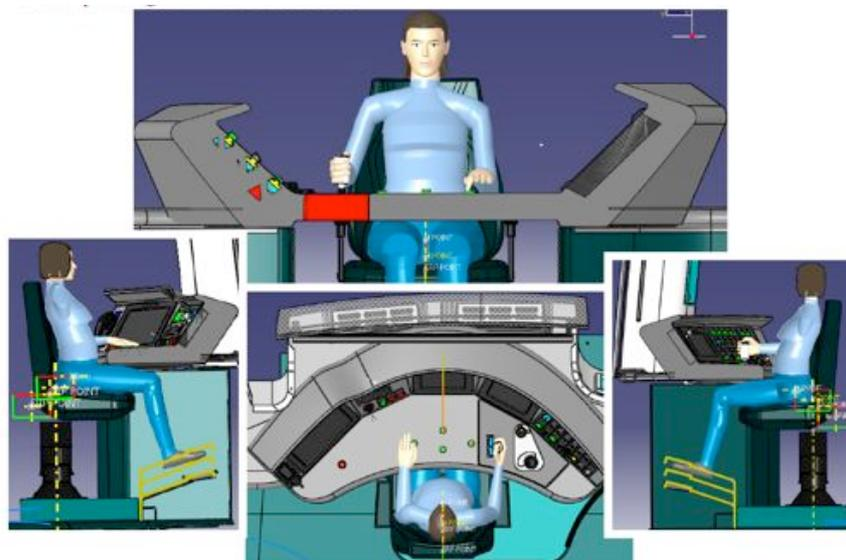
**Figure 4: Body posture for a small woman (1600 mm body stature) in normal driving posture (upper body tilted 10 deg. backward) when operating the master controller and pushing ‘door open’ button**
