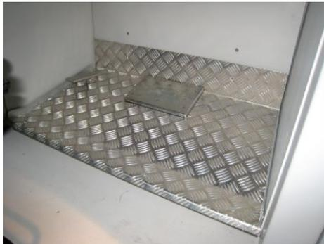
**Figure 5: Adjustable footplate (embossed) with smooth deadman’s pedal just left off centre and actuating pedal top left**
