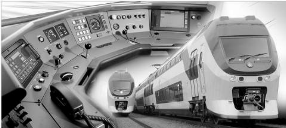
Figure 1. V-IRM trainsets and control table showing the diagnostic screen on the right.
