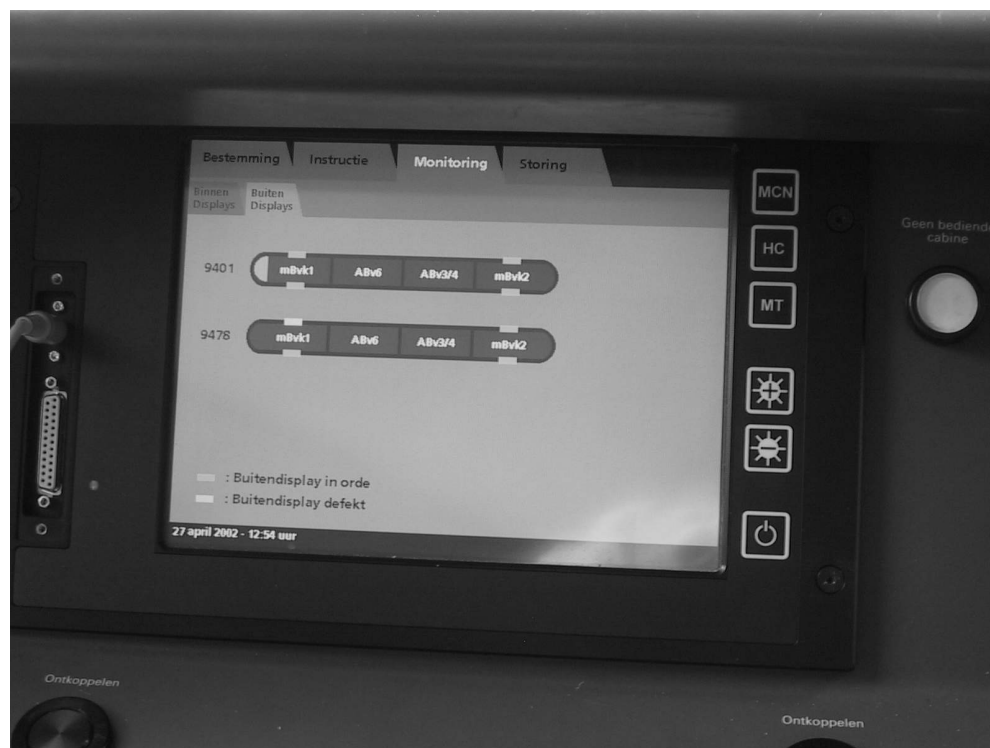
Figure 2. Colour touch screen on the control table in the cabin
